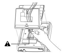
Attach the power adaptor to the base of the telephone where the warning symbol is marked. Connect the power adaptor into the closest electrical outlet.
