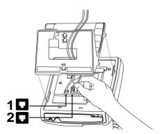
Attach the line cord to jack number 2 and the other end to the modem or fax machine. This line cord is not supplied with the telephone.
