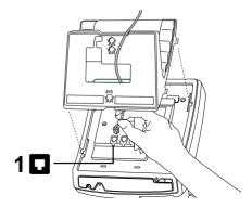
Attach one end of the line cord to jack number 1 and the other end of the line cord to the wall jack.
