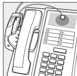
3. Connect the Remote Handset Lifter to your wireless system. Insert the AUX Plug into the large port marked AUX on the base of your wireless headset system (you will need to remove the Stand to access this port).\*
